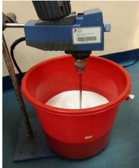
Figure 2. Homogenization Process Using Mechanical Stirrer
