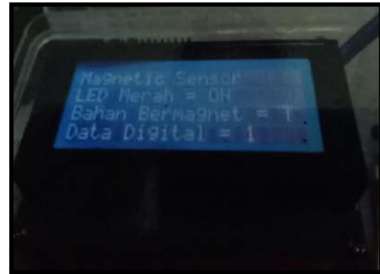
Rajah 10. Paparan bagi Magnetic reed switch module for Arduino
