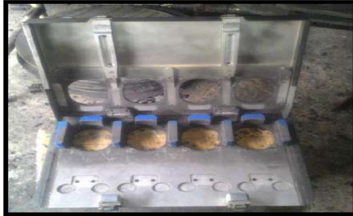
Figure 2. Inner View Of Current Spray Fixture
