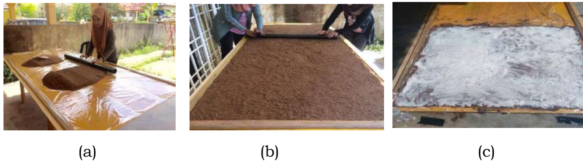
Figure 3. (a) Blended dry leaves compaction, (b) Compaction on the square mould, (c) Compacted dry leaves glues with the latex.
