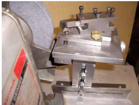
Rajah 3. Tool Grinding Jig Sumber:
