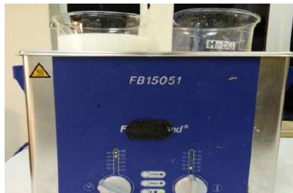
Figure 3. Sonication Process Using Ultrasonic Bath for 2 Hours
